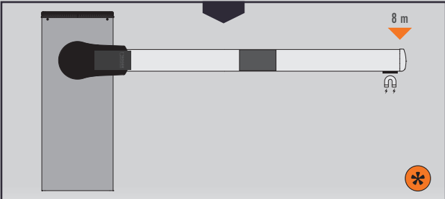
boom with internal joint and magnet
