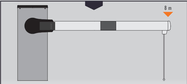
boom with internal joint and rest
