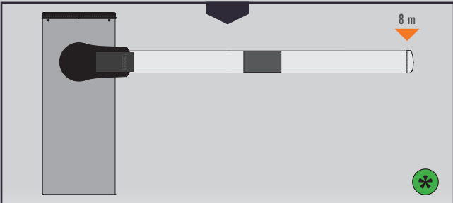
boom with internal joint
